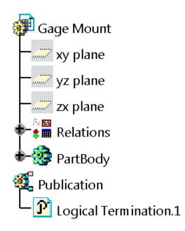
The publication does not necessarily point to a specific element, but instead defines electrical termination properties for the device.
