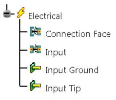
**Create the necessary connector connection points and terminations for the three output connectors.** This will leave the part with all necessary connections and terminations defined.
